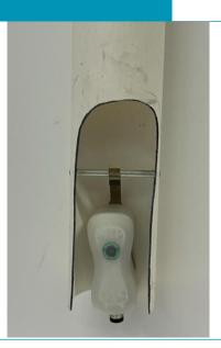
The clip allows the FireFly to be installed with a hook hanging vertically on a wire up to 6 mm in diameter. This clip is used for mounting in the Macro Solar Chimney.
