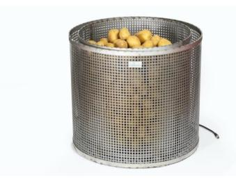
The Potato Guard measures real-time weight loss of seed potatoes during storage. This measurement helps you set climate and ventilation parameters, minimizing mass and quality loss during storage. The Potato Guard is buried at the level of the storage top. An optional lid can be used for deeper measurements.
