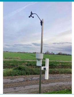
The weather station includes a wind gauge, pluviometer, air temperature and relative humidity. Optional features include a GPS module and a stainless steel pole.
