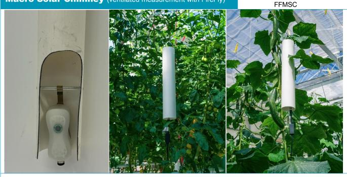
The Macro Solar Chimney is a passively ventilated housing for the FireFly. In environments with high irradiance (direct growth or sunlight), this housing provides a more accurate measurement of temperature and relative air humidity. When using the Macro Solar Chimney, the PAR measurement is not usable because the light sensor is shielded.
