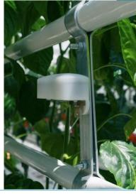
Smart clip for attaching the Firefly against steel or iron objects
