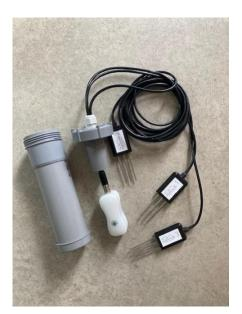
Specially designed for use of Poseidon sensors in public green spaces is the Poseidon City sensor housing. This allows a FireFly with one or more Poseidons to be placed underground and therefore invisible. The housing also provides protection against mechanical and chemical weed control. The photos show a Poseidon Triple City; there is also a version with a single or double Poseidon available.
