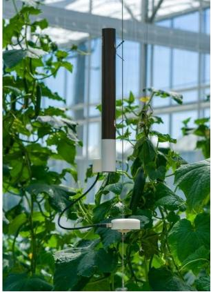
The Solar Chimney TrV is designed for temperature and relative humidity measurements in the presence of high (solar) radiation. The radiation generates natural airflow through the chimney, allowing for ventilated air temperature and relative humidity. The FireFly platform sensor is connected via connector cable and provides data transmission. There are multiple mounting options to choose from. Use the Solar Chimney SubZero model for measurements below 0 °C (upon request).
