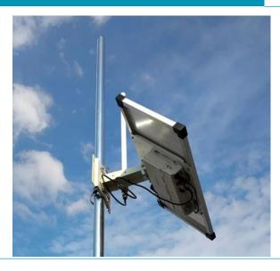
The outdoor 4G gateway receives LoRa messages from the FireFly sensors and sends the data over the Internet to the database. A single gateway is sufficient to process data coming from up to 100 FireFlies. Suitable for outdoor use, this GoutSolar gateway connects via a 4G connection and/or an Ethernet cable.
