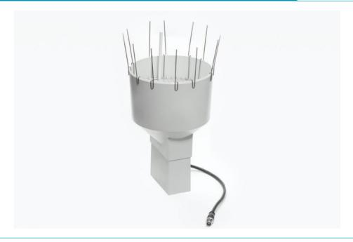
The pluviometer consists of a funnel with anti-bird stings mounted on a "tipping bucket" sensor. The pluviometer measures precipitation in mm, and can be connected to a FireFly.
