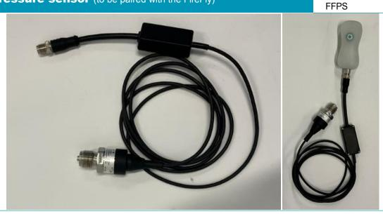
The liquid pressure sensor measures line pressure in, for example, water supply and irrigation systems. The pressure sensor is mounted with a (straight) G 1/2 inch male thread. The pressure sensor is connected to a FireFly.
