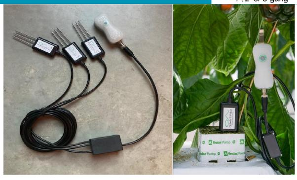
The Poseidon WET sensor measures permittivity, electro-conductivity (EC), and temperature of soil or substrate. Single, dual, and triple versions are available. This makes it possible to monitor transport of water and nutrients through the soil. The (multi-) Poseidon should be connected to a FireFly.
