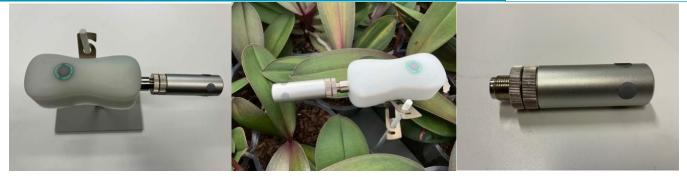
This sensor measures the concentration of  $CO_2$  in the ambient air. The measured concentration is compensated for changes in temperature and air pressure. With a separately supplied calibration kit, the sensor can be easily calibrated by the user himself.
