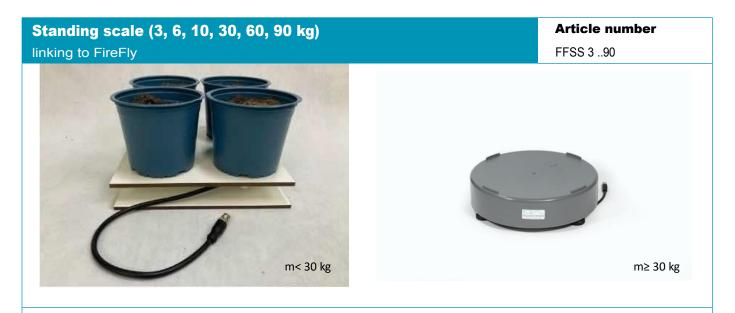
The upright scale can be used for weighing medium to large pots, to support irrigation and/or biomass determination. The scale comes in a square or round design, with a measuring range of 3, 6, 10, 30, 60 or 90 kg. The scale
