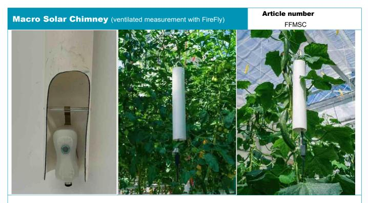
The Macro Solar Chimney is a passively ventilated housing for the FireFly. In environments with high irradiance (direct growth or sunlight), this housing provides a more accurate measurement of temperature and relative air humidity. When using the Macro Solar Chimney, the PAR measurement is not usable because the light sensor is shielded.
