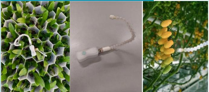
The infrared thermometer allows non-contact measurements of the surface temperature of, for example, plant leaves. The thermometer has a wide measuring range and a high accuracy of up to 0.3 °C. The device is used to detect plant stress.
