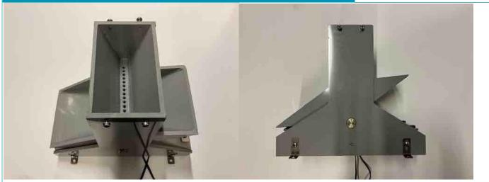
The drain/dripper sensor is a tipping-bucket sensor for measuring large drain volumes. The sensor connects to a FireFly.
