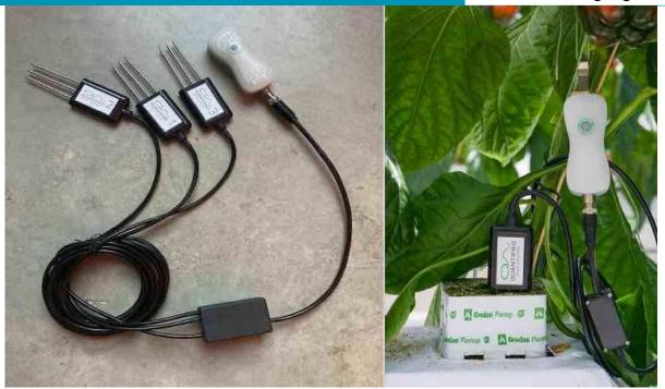
The Poseidon WET sensor measures permittivity<sup>\*</sup>, electro-conductivity (EC), and temperature of soil or substrate. Single, dual, and triple versions are . This makes possible to monitor transport of water and nutrients through the soil. The (multi-) Poseidon should be connected to a FireFly.
