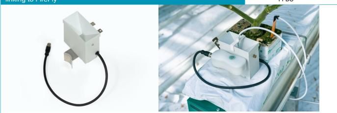
The drain/dripper sensor is a tipping-bucket sensor for measuring drain volume. The sensor is connected to a FireFly.
