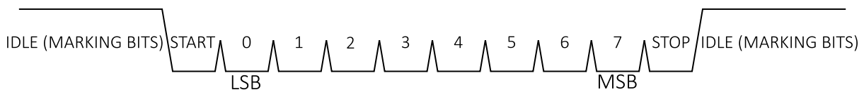
Figure 4: Minimum break character required to wake-up the Slave device.
