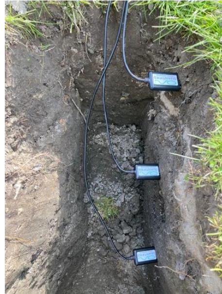
Insert the Poseidon pins firmly in the sidewall
