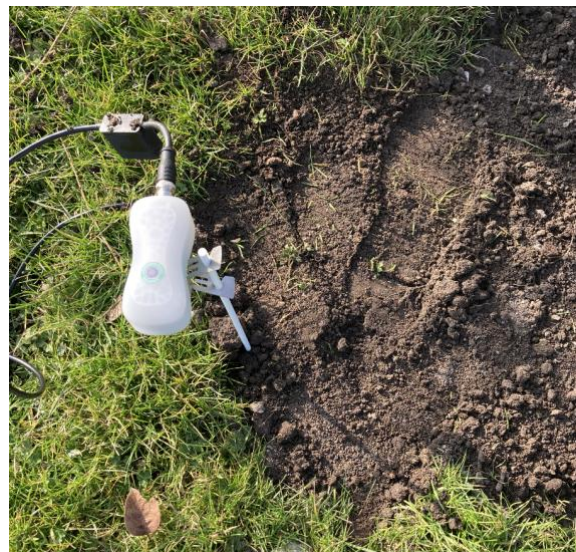
Gently bring back the soil and gently compress till the surface is even.
