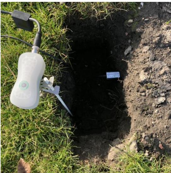
Place the Firefly sensor on the stick
