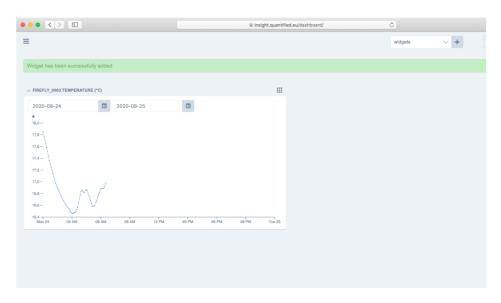
You can Add, Change, Move and Delete Widgets on your Dashboard. To **Add** a Widget from the Widget drop down select a Widget type and click on the +.
