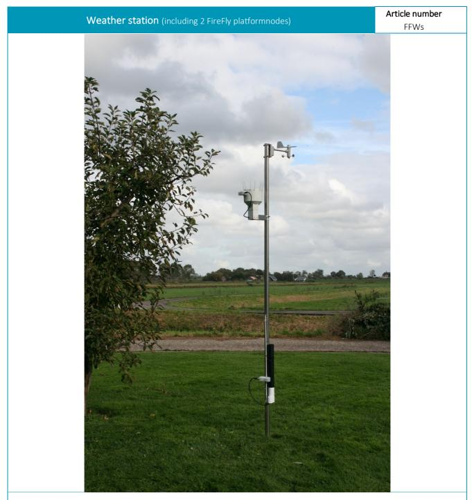
The weather station combines a pluvio meter, windspeed meter, wind direction meter, ventilated air temperature, ventilated relative air humidity, PAR-light, barometric pressure and 2 (50cm and 250cmfrom ground) non-ventilated air temperature and non-ventilated air humidity. Optional a GPS module and a stainless-steel anti-theft pole.
