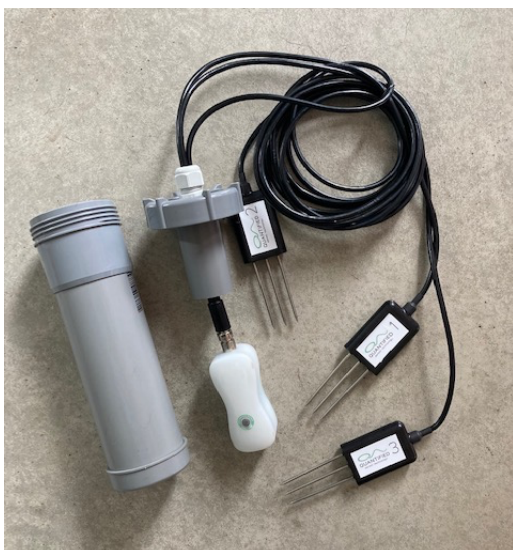
Step 1. Connect the firefly and reset with the magnet (record the sensornumber to match the measurements later on)
