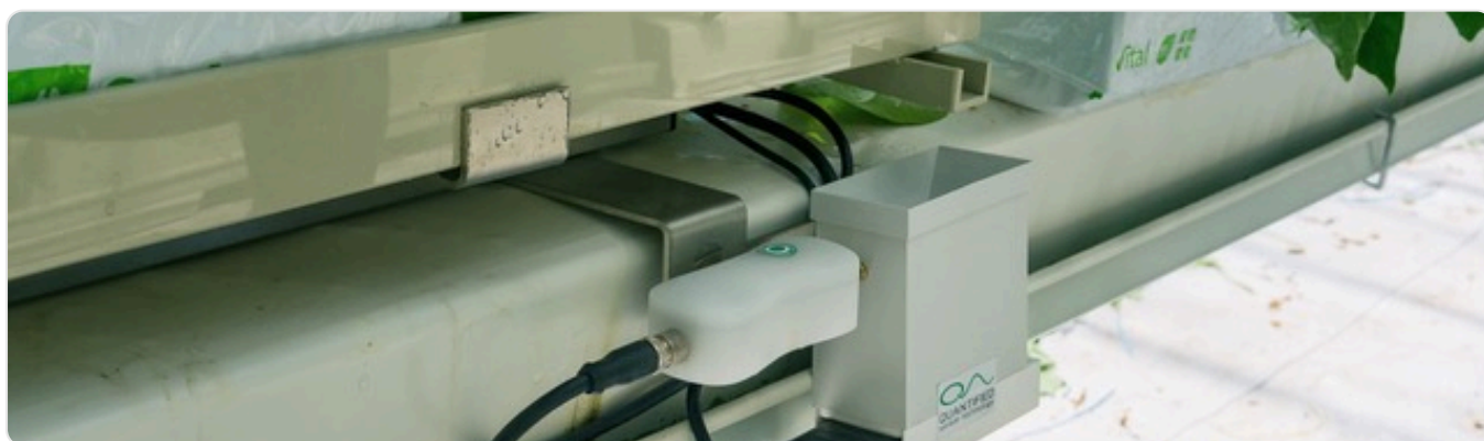
Figure 1. Direction of inclination for drain, the reset spot on the FireFly (LED blinks red, then green) and the drain positioned over the funnel.
