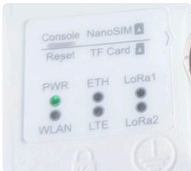
Figure 3. When everything is connected correctly, the power indicator (PWR) on the gateway lights up green .
