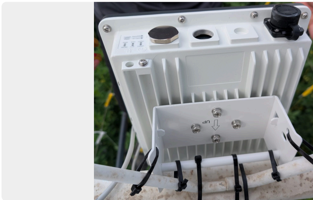
Figure 4. The underside of the gateway should never be exposed to water. Close it off with the tape provided in the box.
